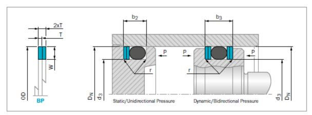
Installation dimensions for the spiral Back-up Ring type, External sealing, material PTFE – Metric
