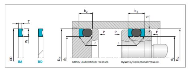
Installation dimensions for concave Back-up Ring types, uncut and cut,
